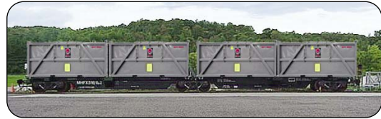
Our high-capacity articulated flat railcars can transport four Shielded Multi-use Type-A containers.
