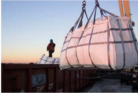
MHF five-yard self-standing bag loading product into a railroad gondola car.
